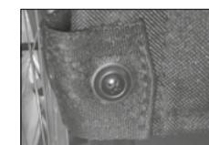
Insert these screws through the grommets on the belt. Reinsert the screws into the screw holes and tighten them.
